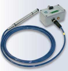
Supply voltage can be monitored internally and is part of the SDI12 measurement response.
