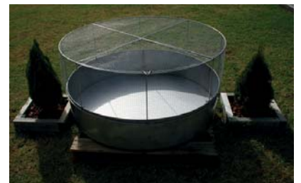
Optional Bird Guard, Measuring Cylinder and Fix Point Gauge with the CAEP
